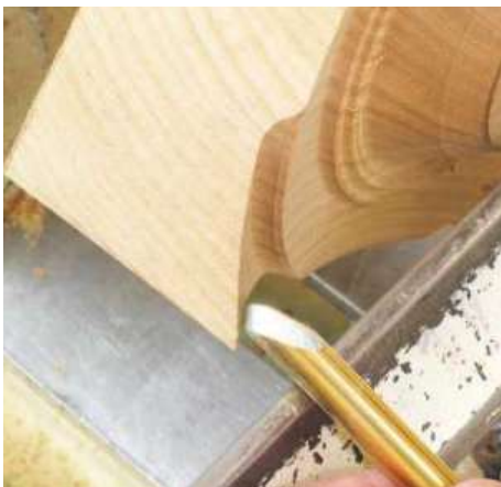
▲ Pic.7 The gouge's angle of presentation is very important. Here I am demonstrating how the bevel is lining up with the direction of the cut
